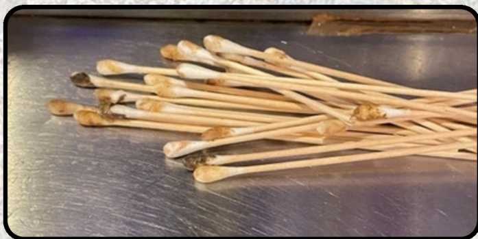
Photo Description: Photo of impacted particles retrieved from the lines connected to taps.
